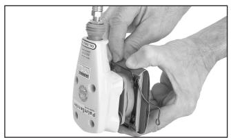
Figure 4. Attaching sandpaper on opposite side.
